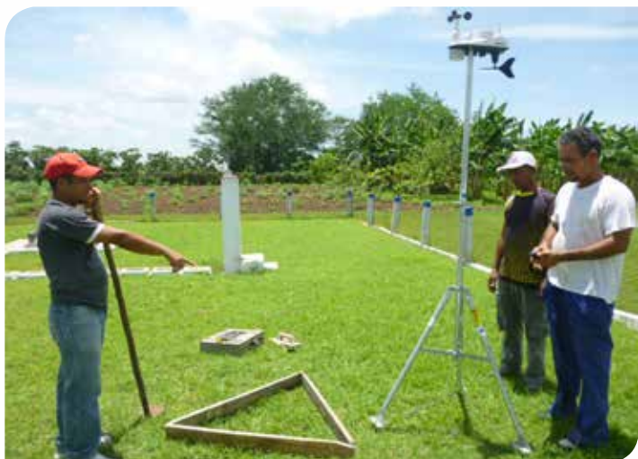
Installation of a portable weather station on a hydrological station operated by volunteer scouts
