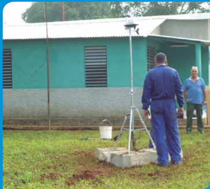
Home in El Pescadero, Cacocum where an Early Warning System radicates which increases its action with the installation of the Davis station, operated by volunteer scouts
